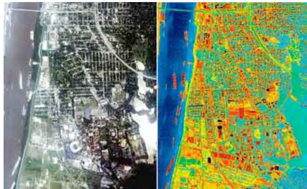
Urban heat island in Baton Rouge, La. (Source: EPA)
